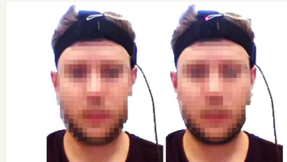
Fig. 9. The LED Indicator used for synchronisation between two tracking systems. Left: Off, Right: On.
